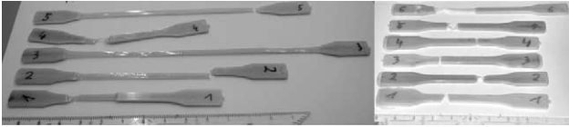
Fig. 8. Tensile samples after testing (left) RP-PBT (right) RP-pCBT.
